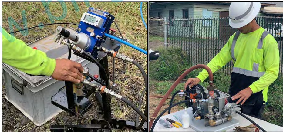
Figure 16 Cable Jetting Machines
