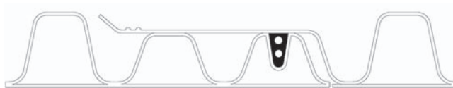
Figure 7.2 Typical Profile Wall Section Showing Bell End (right) and Spigot End (left)
